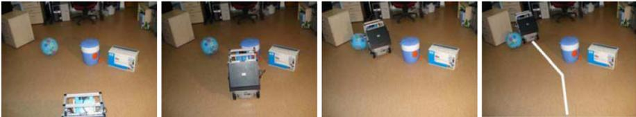
**Fig. 13.** This sequence shows how the perception of traversability affordance are used to navigate in blocked situations. The initial position of the robot is shown in the left-most figure. The robot first goes forward, then turns left since trash-bin does not afford traversability. Third snapshot shows the robot driving over the spherical object. The path of the robot is shown in the last figure. (source: [67]).
