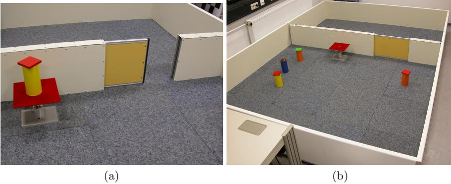
**Fig. 7.** (a) The physical test arena, called demonstrator scenario, including a separating wall, a sliding door, and a (red) switch to open the door. (b) The switch can be operated by putting a weight on it, which will open the door. Removing the weight will close the door. This particular set-up has been chosen to train the robot to observe effects of its manipulation actions.
