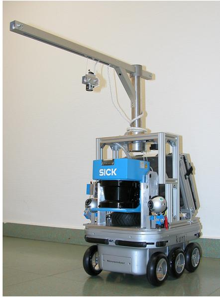
**Fig. 6.** The mobile robot KURT3D, equipped with a crane arm manipulator and a magnetic gripper
