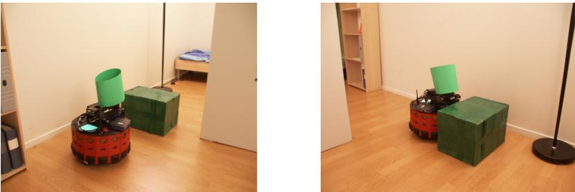
**Fig. 4.** A robot querying and then pushing a PEIS-box through a doorway
